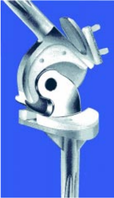
Figure 7. A hinge prosthesis (GSB) with a patellar flange and long stems for intramedullary fixation. Half the femoral component is removed to display the inner design with a PE liner to avoid direct metal to metal articulation.
